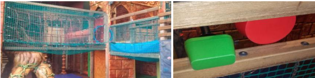
Photograph 3 Application of probes to an item of playground equipment in Slovenia
